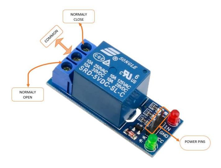
NOTE: whatever was the relay channels number the pinconfiguration is the same for every channel except the power pins (VCC and GND) are for the board itself. The input signal (IN) pin for every relay.
